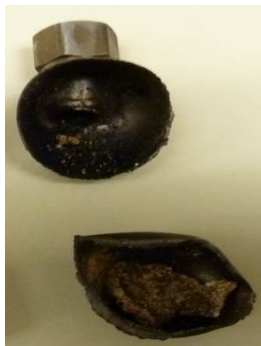
Figure G-5. ARC Bomb after 7.5 g 16 h dried 3.5 M HNO 3 /Swheat Scoop® Experiment
