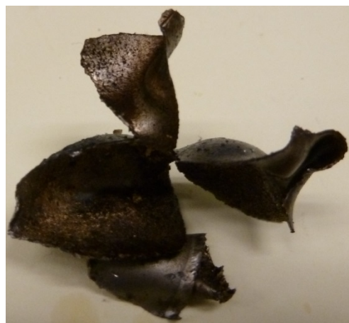
Figure G-6. ARC Bomb after 7 g 7-day dried 3.5 M HNO 3 /Swheat Scoop® Experiment
