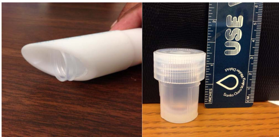
Figure B-2. Delrin ® /Teflon ® sampler, shown with Teflon ® vial in the collector and with Teflon ® vial sealed for sample transport.
