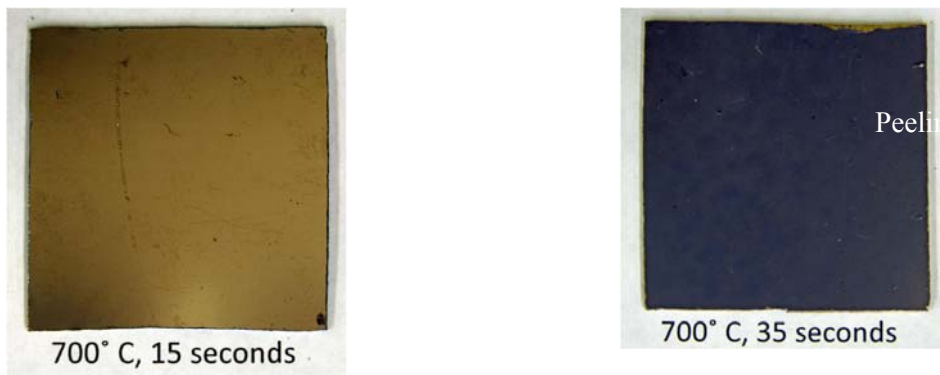
Figure D-30. Metal drum coupons exposed to a temperature of 700C in air.
