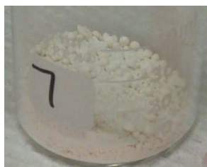
Figure C-24. MgO sample collected from super sack in Panel 7 Room 7.
