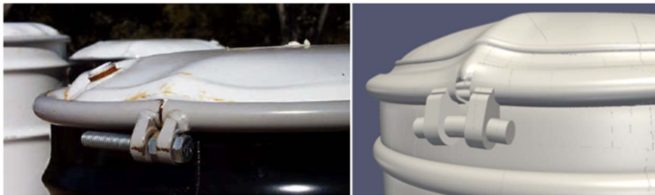
Figure D-15. Comparison of tested drum at LANL (Larranaga et al., 1999) left, and analysis results, right.
