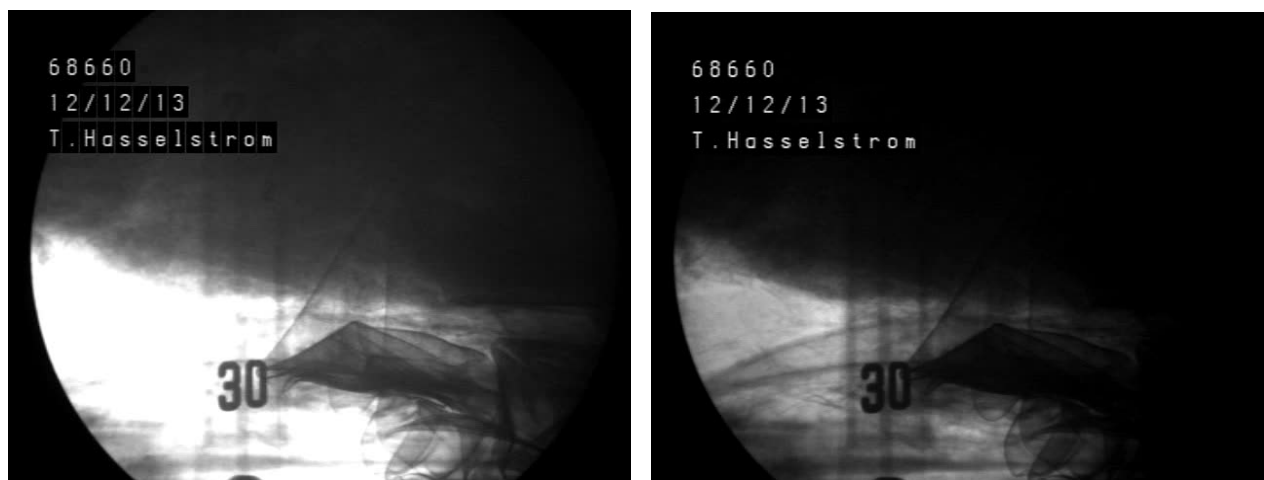
Figure C-12. Radiograph of job control solid waste layer in Drum 68660 showing the glovebox glove
